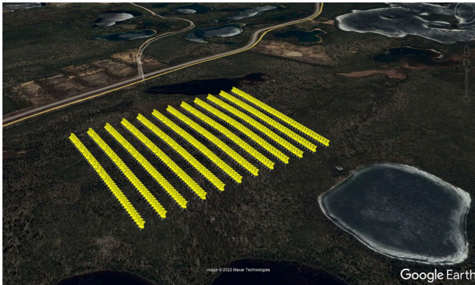
Planned ground gravity stations at Cancet (imagery courtesy of Google Earth).
